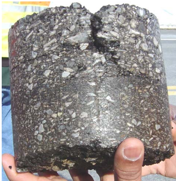
Figure 3 Example of Core Taken from Cracked Section where the STRATA Layer is Still Intact
