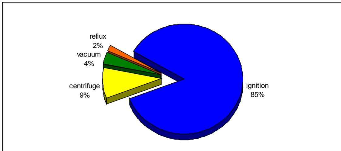
Figure 9. Methods Used to Determining Asphalt Content of RAP Stockpiles.
