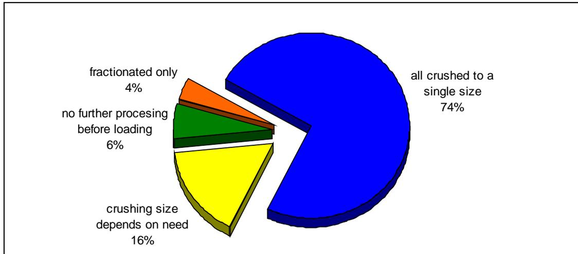
Figure 2. Summary of How RAP is Crushed
