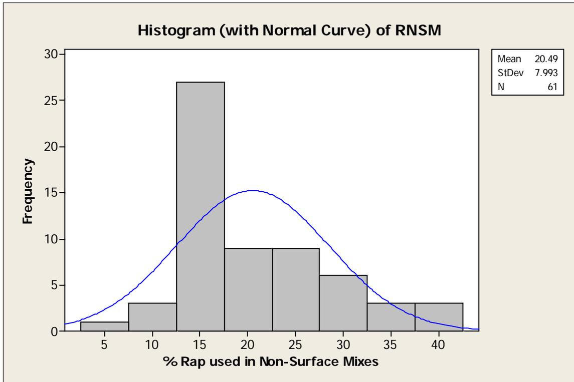
Figure 6. Histogram of % Typical RAP Used in Non-Surface Mixes
